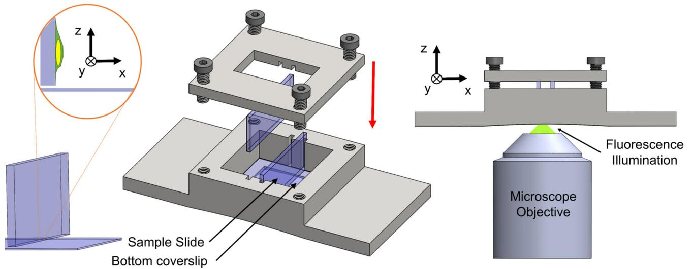
**Figure 1. Schematic of the orthogonal imaging chamber.**
