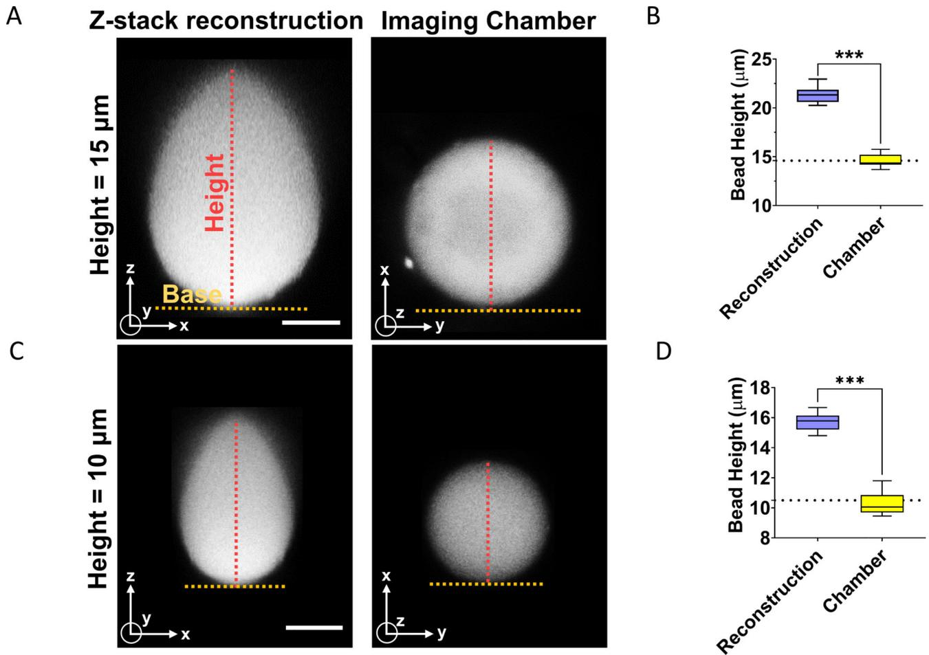
**Figure 2. Comparison of x-z shapes reconstructed from confocal sectioning, and corresponding x-y shapes acquired in the orthogonal imaging chamber.**
